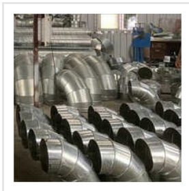
Galvanized Steel Spiral Duct
